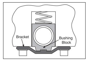
**Figure 36.** Sawdust can get trapped between the bushing block and the bracket.
